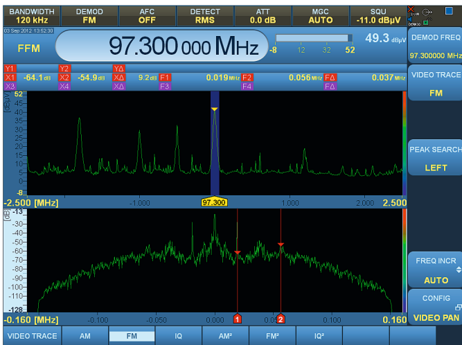
Display of the subcarriers of an FM radio signal using an FM-demodulated video spectrum (pilot tone: 19 kHz; RDS signal: 56 kHz from center frequency).
