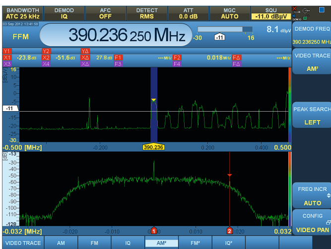
Transmission rate estimate of a TETRA signal using a squared video spectrum (signal peaks approx. 18 kHz from center frequency; transmission rate approx. 18 kBd).
